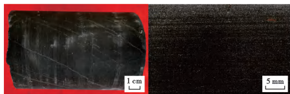
(a) 灰黑色硅质页岩,发育极薄纹层,S1岩相,L214井4287.71 m
